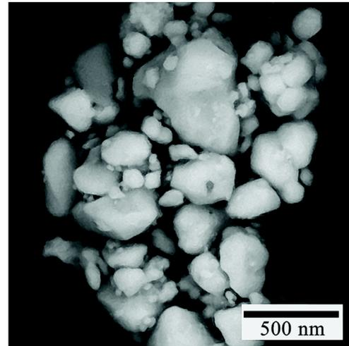
Fig. 6. Backscattered image of the PZT powders hot-milled for 6 h at 800 °C.
