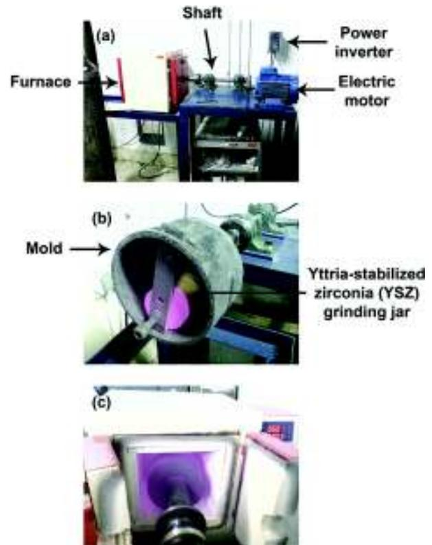
Fig. 1. Pictures of the designed hot milling setup; (a) the whole setup consisted of furnace, electric motor, shaft, digital inverter, etc. (b) the zirconia jar affixed to the steel mold, and (c) the grinding media inserted into the high temperature furnace.
