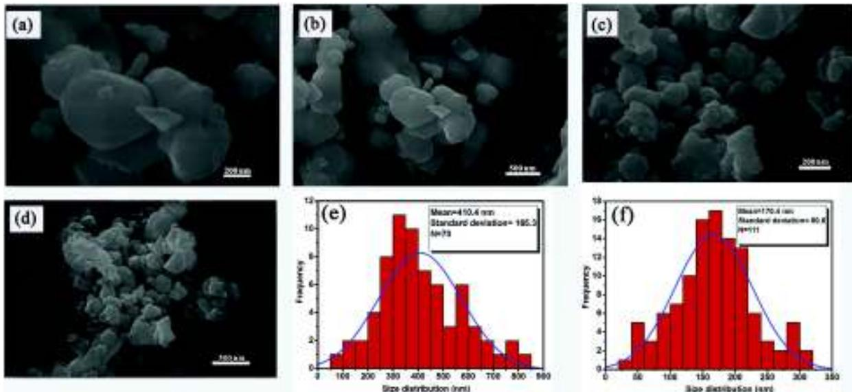
Fig. 5. FE-SEM micrographs of the obtained PZT powder after milling at 800 °C for (a, b) 6 h and (c, d) 12 h at two different magnifications. Particle size distribution of the PZT powders synthesized for (e) 6 h and (f) 12 h.
