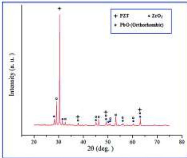
Fig. 4. X-ray diffraction pattern of the obtained powder after hot milling at 700 °C for 36 h.
