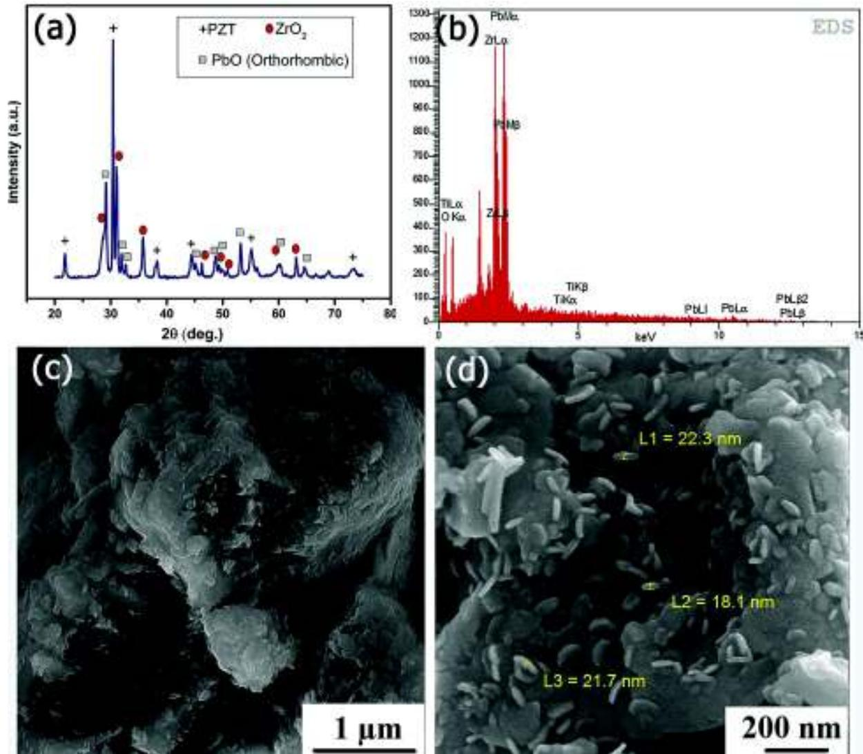
Fig. 7. (a) XRD pattern of the obtained powders by conventional solid-state technique, (b) EDS analysis and (c, d) FESEM micrographs of the synthesized powders.
