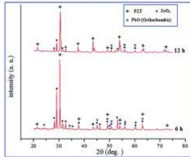
Fig. 3. X-ray diffraction patterns of the synthesized powders after hot milling at temperature of 700 °C for 6 and 12 h.
