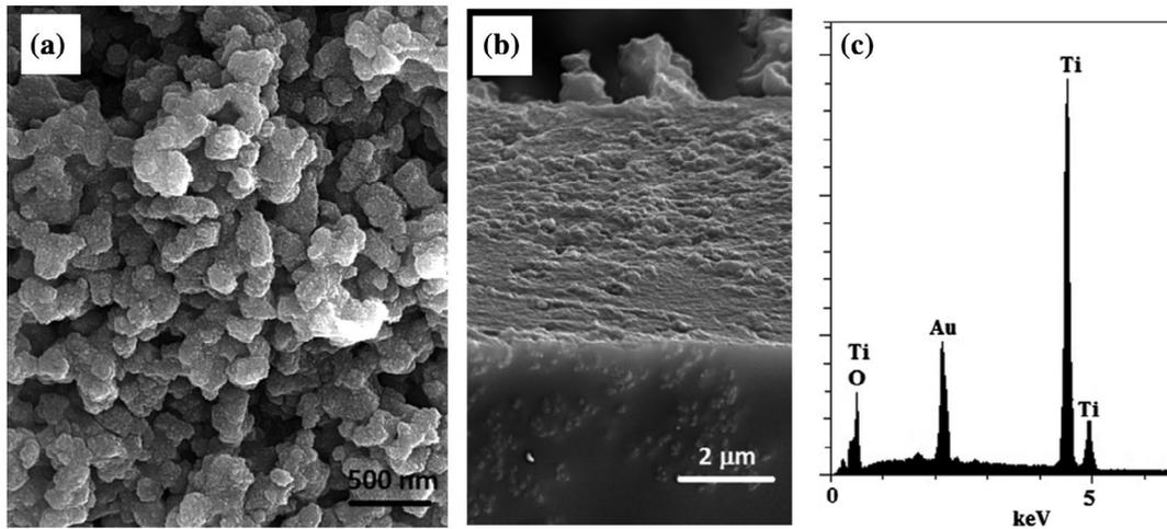
Fig. 5. TiO<sub>2</sub> network sample: (a) SEM image, (b) cross section image and (c) EDS diagram.
