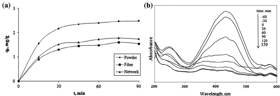
Fig. 6. (a) Adsorption kinetics of MeO on TiO<sub>2</sub> geometries in the dark and (b) changes in the UV-vis spectra during photodegradation of methyl orange on TiO<sub>2</sub> powder.
