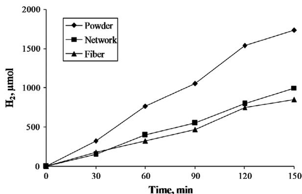
Fig. 9. Effect of TiO<sub>2</sub> geometry on H<sub>2</sub> generation activity from 50 vol.% methanol solution.
