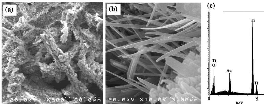
Fig. 4. TiO<sub>2</sub> fiber: (a) and (b) SEM image and (c) EDS diagram of fibers.
