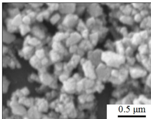
Fig. 5. Micrograph of the nickel oxide nano-powder produced via rapid microwave-assisted route.
