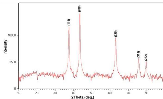
Fig. 3. XRD pattern of the nickel oxide powder produced in this research.
