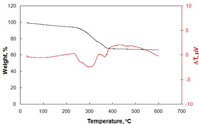
Fig. 2. STA (TG/DTA) graphs of nickel hydroxide. Experimental conditions were: (a) 1min holding at  $30^\circ\text{C}$ , (b)  $10^\circ\text{C}/\text{min}$  temperature raise from 30 to  $600^\circ\text{C}$  and (c) 10min holding at  $600^\circ\text{C}$ .
