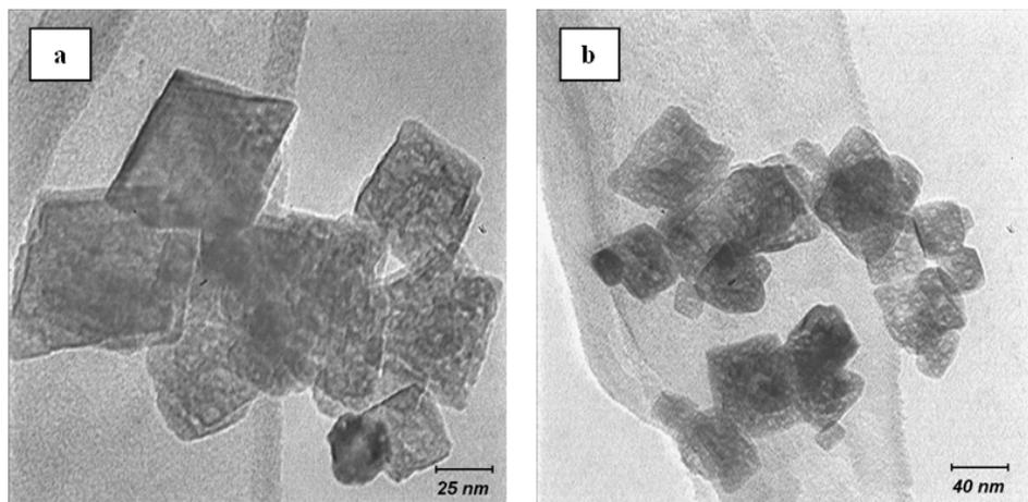
Fig. 6 Transmission electron micrograph of NiO nano-powder synthesized via rapid microwave-assisted route.
