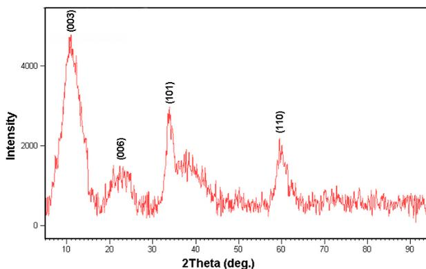
Fig. 1. X-ray pattern of nickel hydroxide powder produced via microwave assisted rout.
