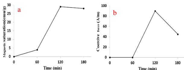
Fig. 4. Changes in specific saturation magnetization with the degree of calcination time (a) and changes in coercivity with the degree of calcination time (b).
