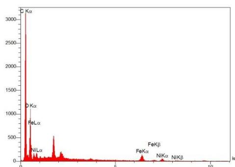
Fig. 2. EDS analysis of  $\text{NiFe}_2\text{O}_4$  nanoparticles in figure 1 (b)
