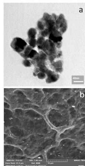
Fig. 1. SEM image of pure  $\text{NiFe}_2\text{O}_4$  nanoparticles (a) and FESEM image of  $\text{NiFe}_2\text{O}_4$  - chitosan (b)
