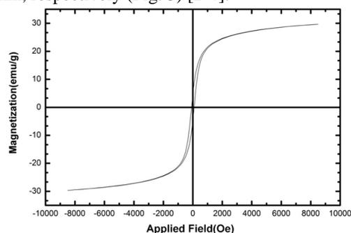
Fig. 3. The magnetic properties of  $\text{NiFe}_2\text{O}_4$  - 2h of calcinations
