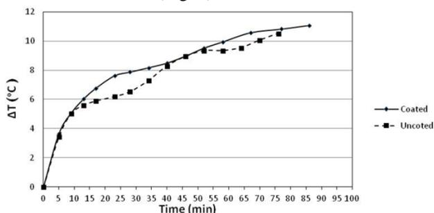
Fig. 5. Temperature increase of pure NiFe<sub>2</sub>O<sub>4</sub> nanoparticles after 2 hours of calcination and NiFe<sub>2</sub>O<sub>4</sub> - chitosan nanoparticles as a function of time
