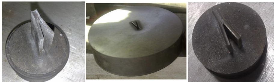
Fig.2- Three pieces powder metallurgy die made from 2714 steel
