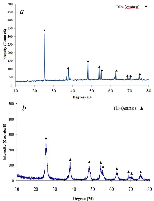
Fig.2: XRD patterns of a)NTT and b)NP TiO<sub>2</sub>
