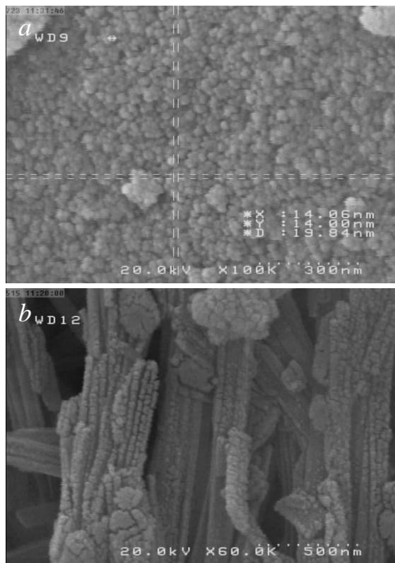
Fig.1: FE-SEM images of surface morphology of TiO<sub>2</sub> a)NP b)NTT
