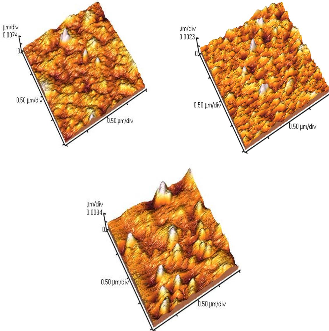
**Fig. 1** AFM images of (a) Fe-Ni, (b) Fe-Co, and (c) Fe-Ni/Fe-Co multi layered thin films fabricated by EBPVD
