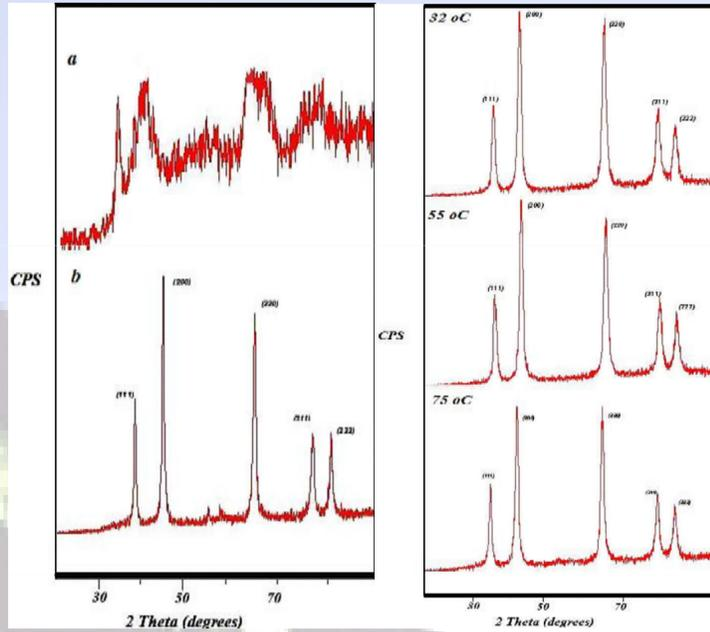
Fig 1. X-ray diffraction spectrum of the nanopowder sample produced by TSSC method: (a) as dried precipitates and (b) precipitate after calcination. The patterns on the right-side indicate the effect of temperature on the calcined product.
