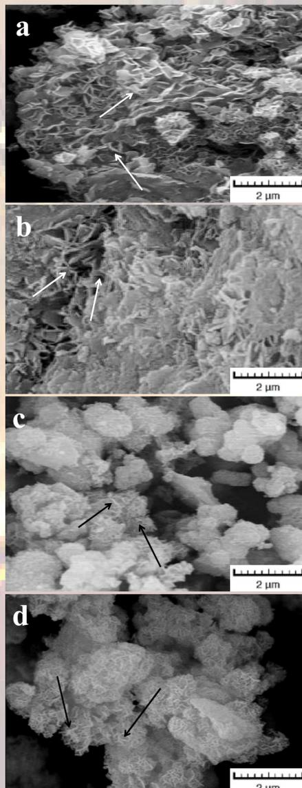
Fig 2. SEM micrograph of the NiO powder synthesized by the TSSC at: (a) 22, (b) 32, (c) 55, (d) 75 degrees Celsius. The arrows highlight wall-shaped NiO nanoparticles.
