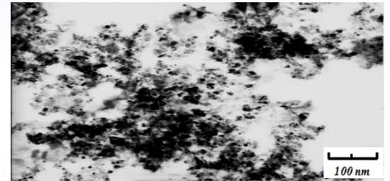
Fig 3. TEM micrograph of the NiO nanopowder produced by the TSSC method at the room temperature.
