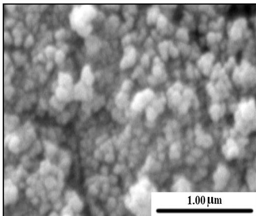
Fig. 4 Micrograph of nickel oxide nano-powder.
