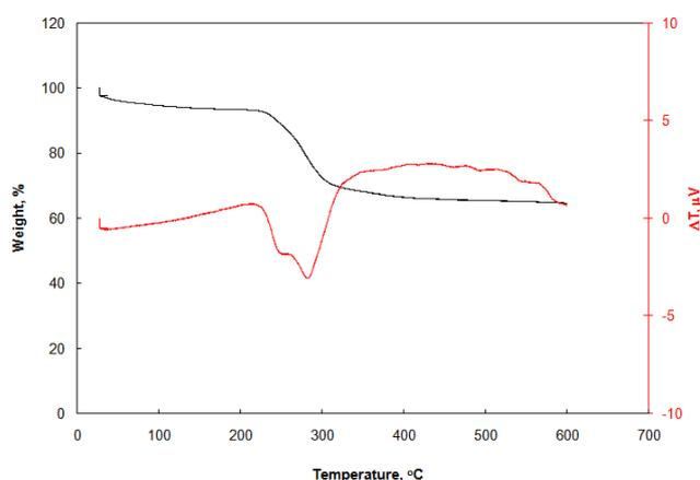
Fig. 2. STA (TG/DTA) graphs of nickel hydroxide; Conditions: hold for 1 min at  $30^\circ\text{C}$ ; heat from  $30^\circ\text{C}$  to  $600^\circ\text{C}$  at the rate  $10^\circ\text{C}/\text{min}$ ; hold for 10 min at  $600^\circ\text{C}$ .
