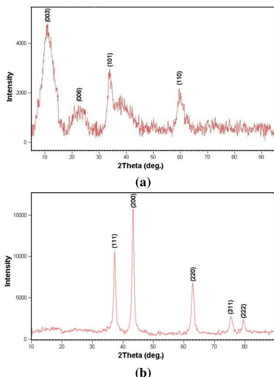
Fig. 1. X-ray pattern of nickel hydroxide powder (a) before and (b) after calcination.
