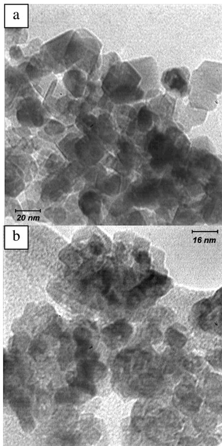
Fig. 5 Transmission electron micrograph of nickel oxide nano-powder.
