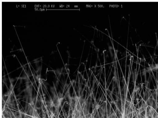
**Fig. 4.** SEM image of SnO<sub>2</sub> nanostructures synthesized under the flow of Ar gas
