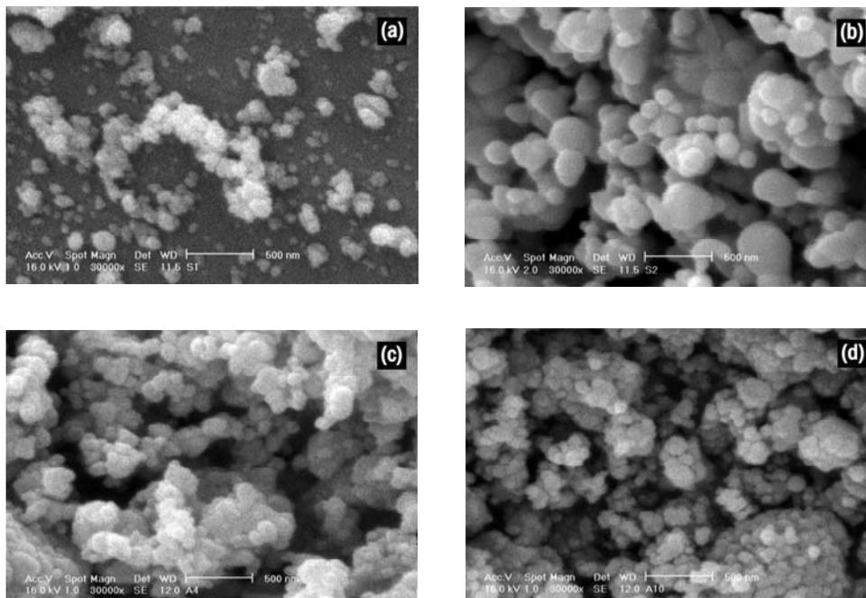
Fig. 2. SEM images of the samples: (a) milled for 20 h, (b) milled for 20 h then annealed at 750°C for 2 h, (c) milled for 20 h then annealed at 750°C for 2 h with NaCl:CoFe<sub>2</sub>O<sub>4</sub> ratio of 4:1 and (d) milled for 20 h then annealed at 750°C for 2 h with NaCl:CoFe<sub>2</sub>O<sub>4</sub> ratio of 10:1.
