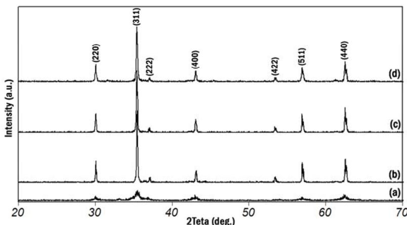
Fig. 1. X-ray diffraction pattern of the samples: (a) milled for 20 h, (b) milled for 20 h then annealed at 750°C for 2 h, (c) milled for 20 h then annealed at 750°C for 2 h with NaCl:CoFe<sub>2</sub>O<sub>4</sub> ratio of 4:1 and (d) milled for 20 h then annealed at 750°C for 2 h with NaCl:CoFe<sub>2</sub>O<sub>4</sub> ratio of 10:1.
