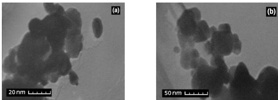
Fig. 3. TEM images of the samples: (a) milled for 20 h, (b) milled for 20 h then annealed at 750°C for 2 h with NaCl: CoFe<sub>2</sub>O<sub>4</sub> ratio of 10:1.
