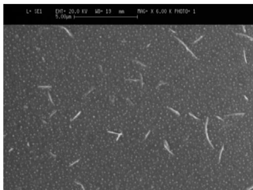
Fig. 7. SEM image of the nanostructures grown on the substrate at distance 5cm away from source materials.
