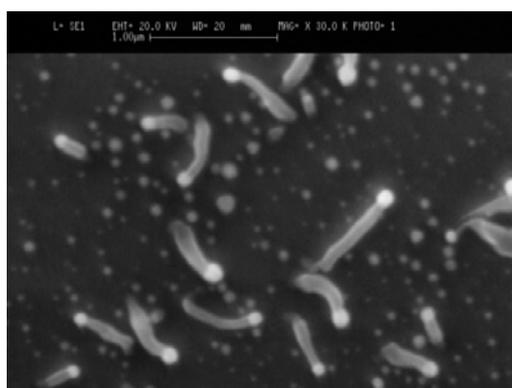
Fig. 1. SEM image of SnO<sub>2</sub> nanostructures grown with SnO<sub>2</sub>: C ratio of 1:1.
